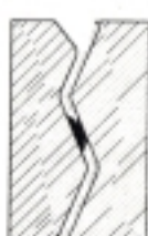
Matoro ® -Drain and Matoro ® joint width: 4mm
