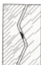
Matoro ® joint width: 3mm
