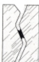
Matoro ® -Drain joint width: 5mm
